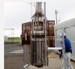
Liquid hydrogen booster pump
