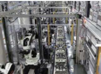
Automated dry vacuum pump assembly line
