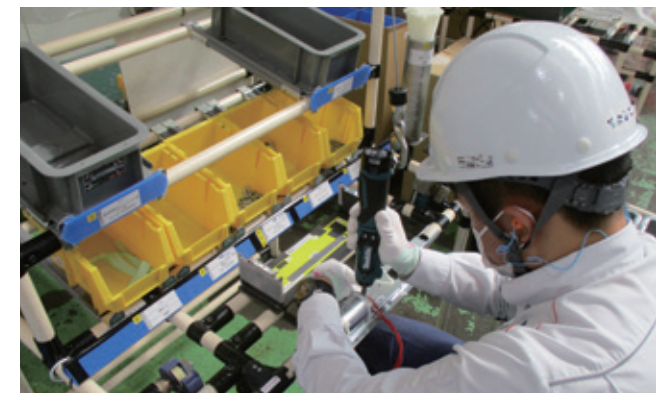
Parts assembly work using electric screwdrivers to install electrical components
